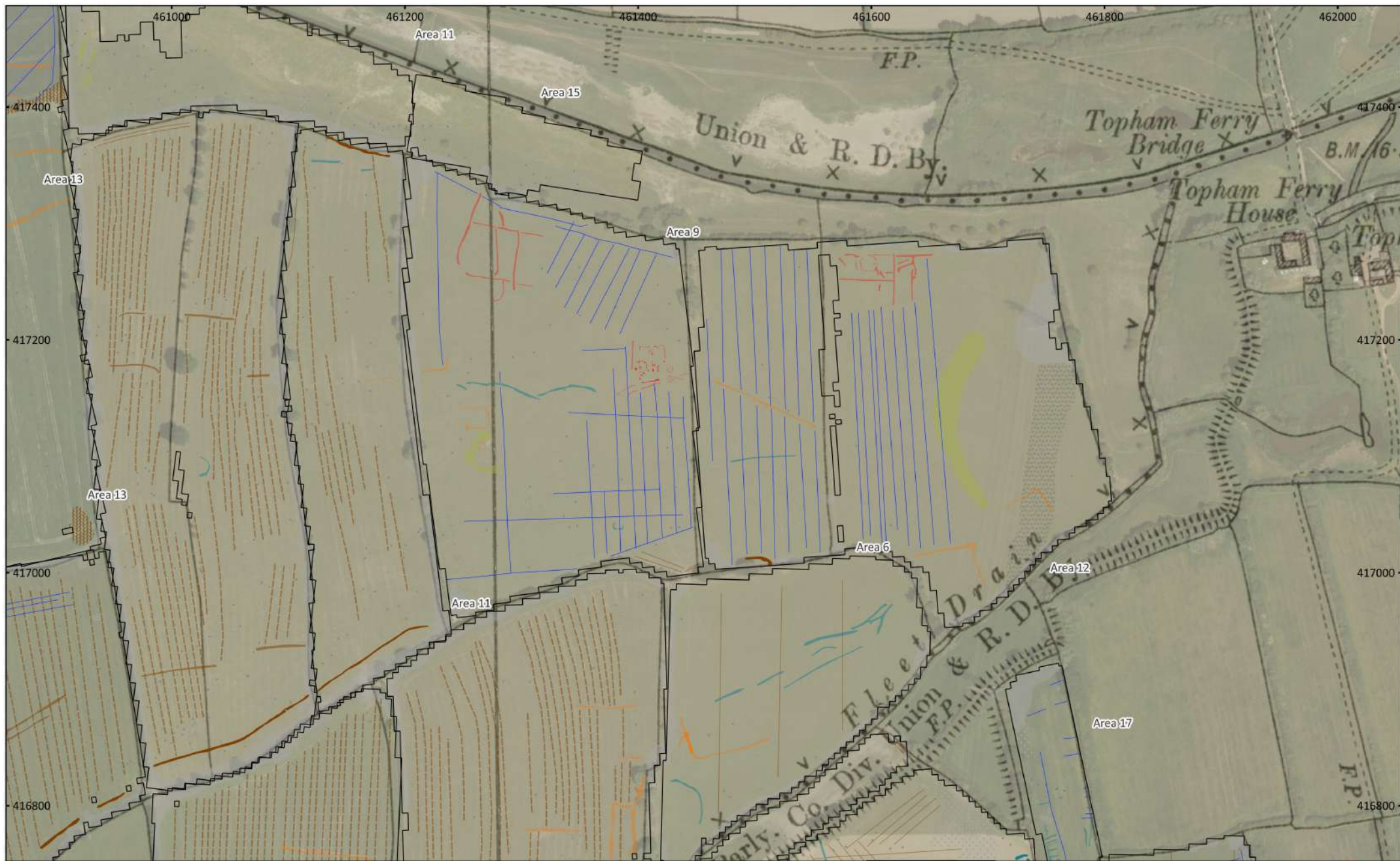
MSSE1569 - Fenwick Solar Farm Scheme, Doncaster Figure 11 - Magnetic Interpretation Over Historical Maps and Satellite Imagery (Northeast) 1:3,000 @ A3 Copyright Magnitude Surveys Ltd 2023 Contains historical mapping © CLS Data 2023: Ordnance Survey, 6" 2nd edition c. 1882-1913 Contains satellite imagery © Bing Satellite 2023
